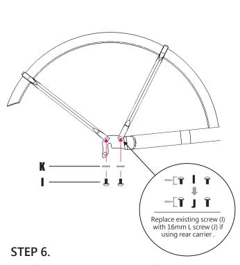
Install fender struts (D) and (E) onto the frame dropout and secure with screw (I) and washer (K). Repeat for other side.
